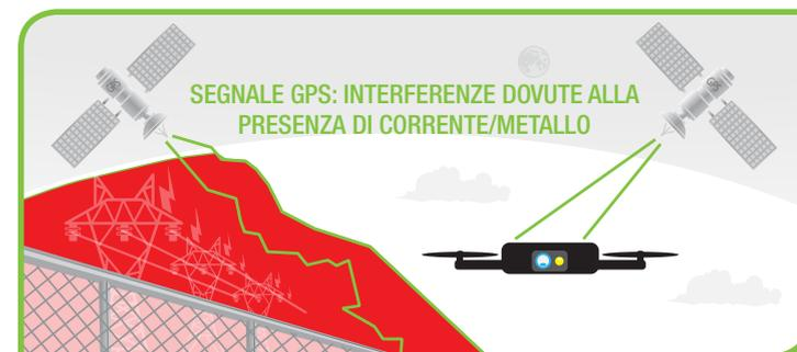
SEGNALE GPS: INTERFERENZE DOVUTE ALLA PRESENZA DI CORRENTE/METALLO
