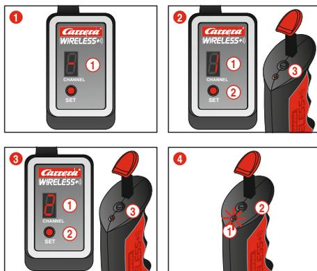
Before the speed controller can be used to control the cars, it must be "bound" to the receiver. To do this, switch on the control unit.
