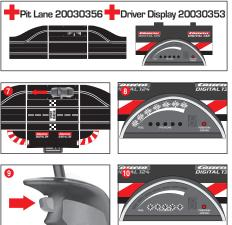
The car's present tank capacity can be read via the bar display with 5 green and 2 red LEDs at the Driver Display. For refuelling drive your car into the Pit Lane across the refuelling sensor fig. **7**. The bar display now starts to flash, fig. **3**, and the car can be refuelled by keeping the lane-change button pushed, fig. **9**. The number of refuellings are indicated by flashing or lighting of the yellow LEDs, fig. 10 (also see Driver Display).
