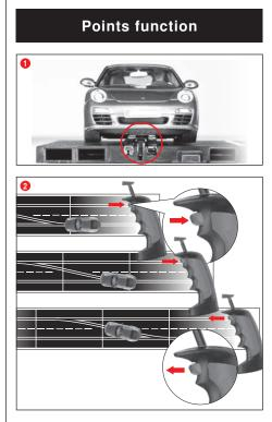
Make sure that the car's guide keel is located inside the track slot and that the double sliding contact is in contact with the current carrying track.
