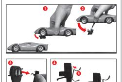
In case the car is lifted, the rocker bar folds up slightly (fig. 1).
