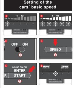
The setting of the basic speed can be effected individually for one and/or several cars. The cars which are to be adjusted have to be positioned on the track. The setting can be carried out on 10 levels with the 5 LEDs indicating the different levels by flashing or permanent lighting.
