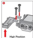
Adjusting the central magnet If required, the central magnet can also be adjusted. Remove the magnet unit from the chassis in its entirety **1**, turn it horizontally by 180 degrees **2** and return it to the chassis. Then mount the magnet retainer (3) and restore all plug connections.
