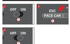
To restore the Control Unit to factory settings the Control Unit offers a reset function.
