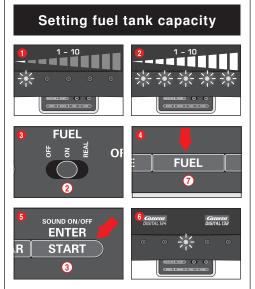
(only for cars operated with speed controllers) The setting of the fuel tank capacity in combination with the Pit Lane (20030356) is effected for all cars simultaneously. The setting can be carried out on 10 levels with the 5 LEDs indicating the different 1 LED lights = low fuel capacity
