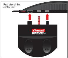
Additional wired speed controllers may be plugged into connectors 3 and 4. Please note that these will use address 5 and 6 then.
