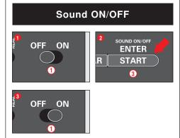
The confirmation sound when crossing the sensors and the key sound can be switched off. Switch off the Control Unit and keep the "START/ENTER" button (3) pushed, switch on the racetrack and release "START/ENTER" (3) again. The acknowledgement sound for switching on the Control Unit cannot be switched off however.
