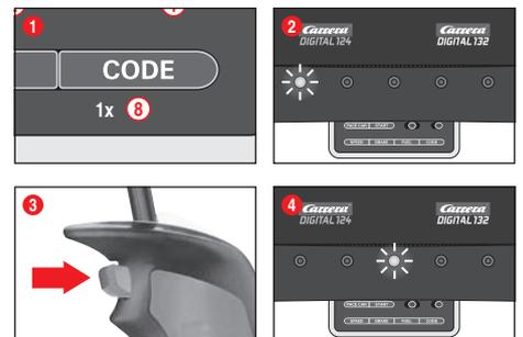
To encode a car place it on the track and switch on the Control Unit. Press "Code" button once 8, fig. 1; the first LED starts to light, fig. 2. Then push lane-change-button once on the relevant speed controller, fig. 3. In case the car is equipped with lights they will start to flash and the Control Unit's LEDs 2-4 will light successively. Once encoding has been carried out the middle LED lights permanently (fig. 4) and the car is allocated to the speed controller.
