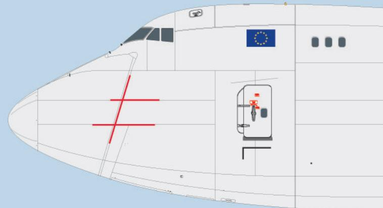
**4. Apply masking tape\* to fuselage**
